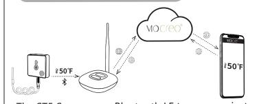
The ST5 Sensors use Bluetooth LE to communicate with the Hub. Therefore, the distance are limited to a Bluetooth range centered on the Hub(e.g., around the house).
